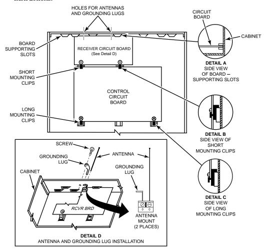
Figure 3. Mounting the PC Board and RF Receiver Together in the Cabinet
