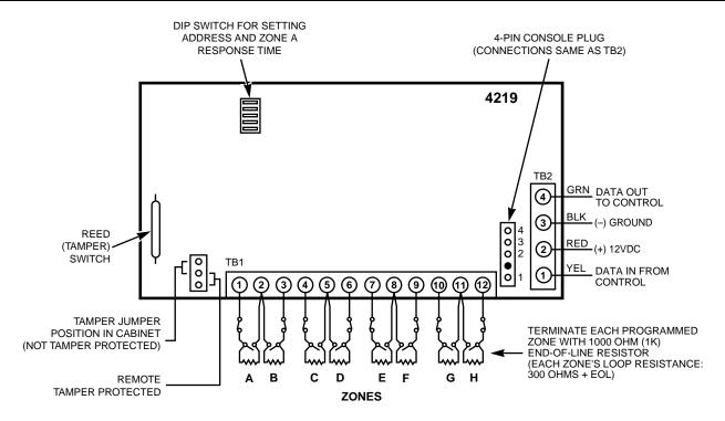
Figure 10. Wiring Connections - 4219 Expansion Module
