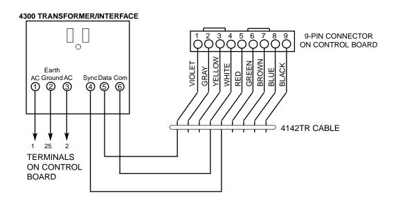
Figure 5. Connections of 4300 Transformer to the Control Board
