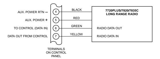
Figure 19. Long Range Radio Connections
