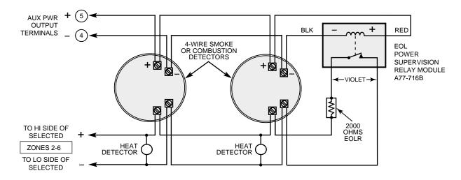
Figure 9. 4-Wire Smoke Detector Connections (Zones 2-6)
