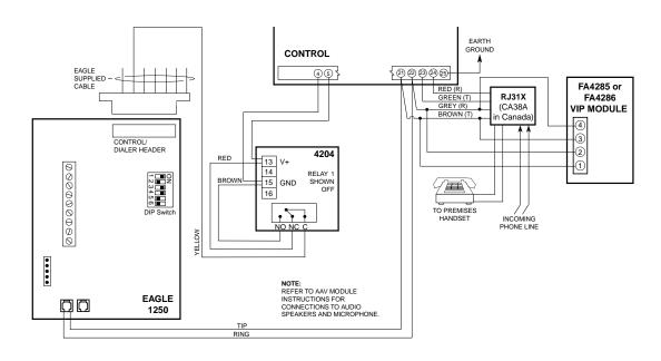
Figure 21. Connection of AAV Unit When Also Using a FA4285 or FA4286 VIP Module
