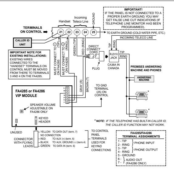
Figure 16. FA4285/FA4286 VIP Module Wiring Connections
