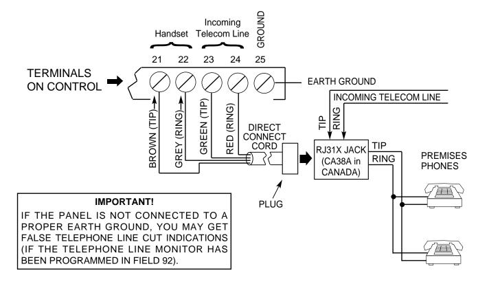
Figure 4. Telephone Line Connections
