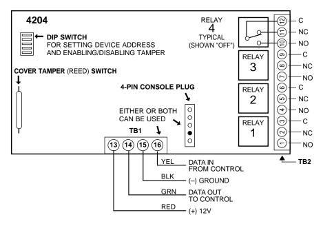
Figure 14. 4204 Connections to Control Panel
