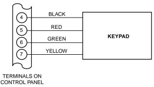
Figure 6. Keypad Connections to the Control Board
