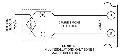
Figure 8. 2-Wire Smoke Detector Connected to Zone 1
