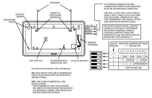
Figure 12. 5881/5882 RF Receiver (cover removed)
