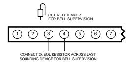
Figure 18. Bell Supervision Wiring
