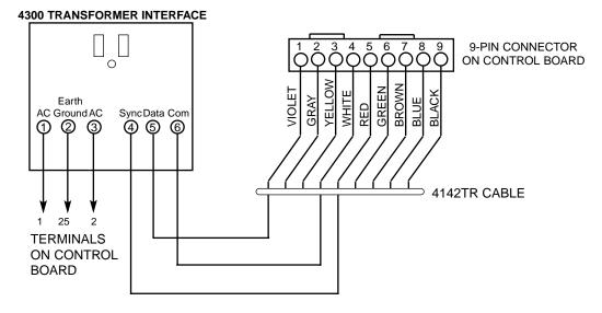
Figure 15. 4300 Transformer Wiring Connections
