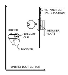
Figure 1. Installing the Cabinet Lock
