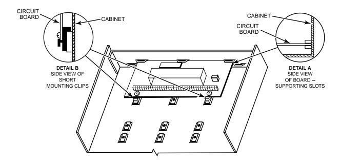
Figure 2. Mounting the PC Board
