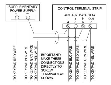
Figure 7. Using a Supplementary Power Supply for Keypads
