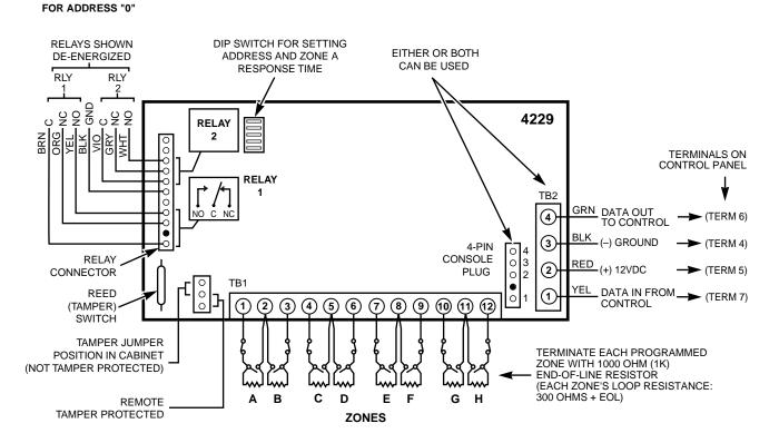
Figure 13. 4229 Connections to Control Panel
