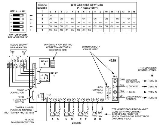
Figure 11. Wiring Connections - 4229 Expansion/Relay Module
