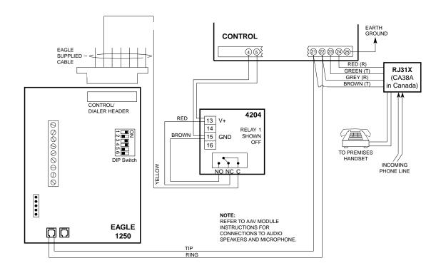
Figure 20. Connection of AAV Unit When Not Using a FA4285/FA4286 VIP Module
